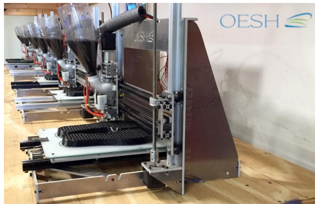
Current OESH 3D printers printing Athena Sandals
