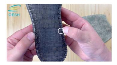
Stitch through the edge of the sole, then through the first marked hole of the fabric.
