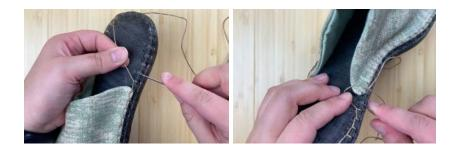
20. Double knot the two thread ends together
