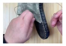
21. For a more secure finish, thread the 2 end strands under a stitch then through to the inside of the shoe, and knot. Trim both ends
